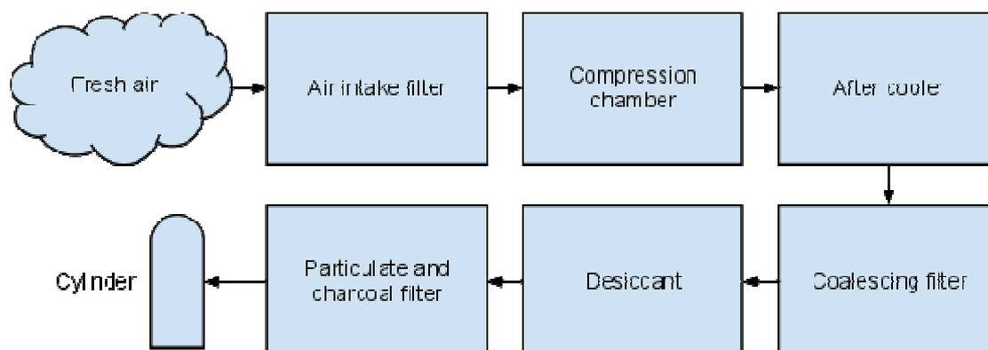
Figure 1 - A typical air compressor system.
